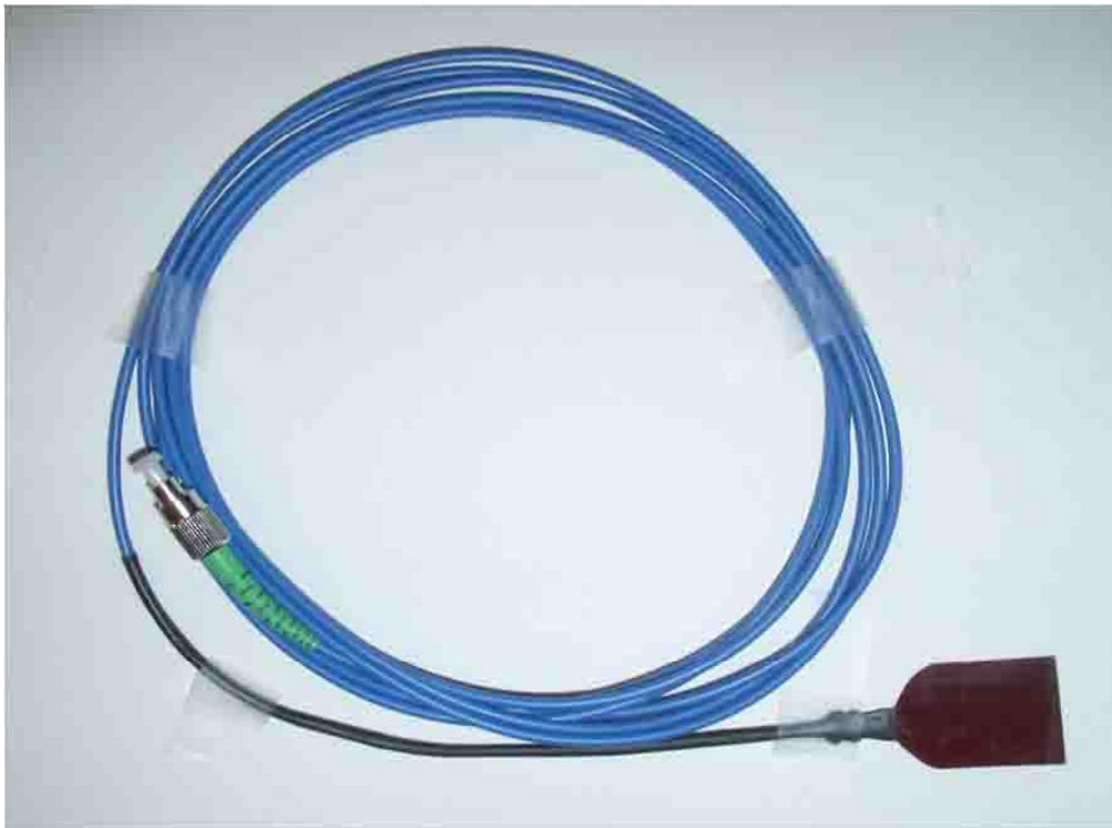
Fig. 5 Picture of the vibration sensor head , 15mm by 10mm Courtesy of QPS
