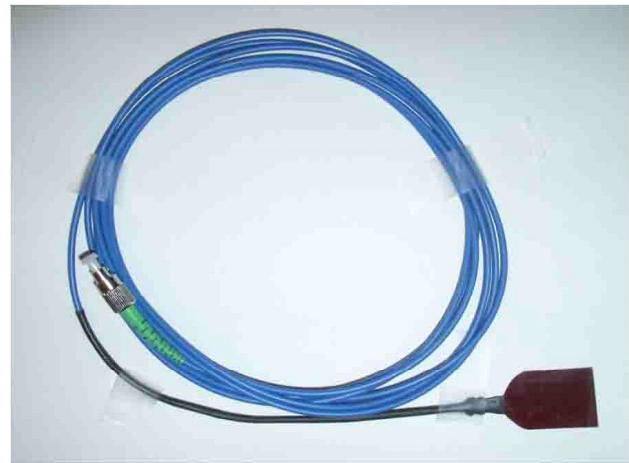
Figure 1. Picture of the vibration sensor head, 15mm by 10mm Courtesy of QPS
